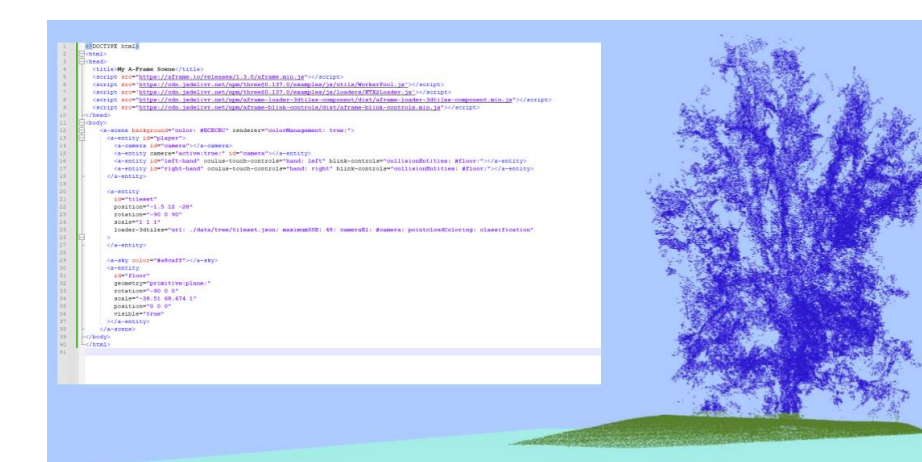
A point cloud converted to 3dtiles via Cesium ion and rendered using A-Frame.
