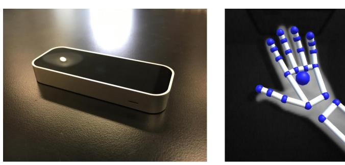
LeapMotion: making use of infrared cameras and complex algorithms to generate the location of arms/hands/fingers in a 3D space.
