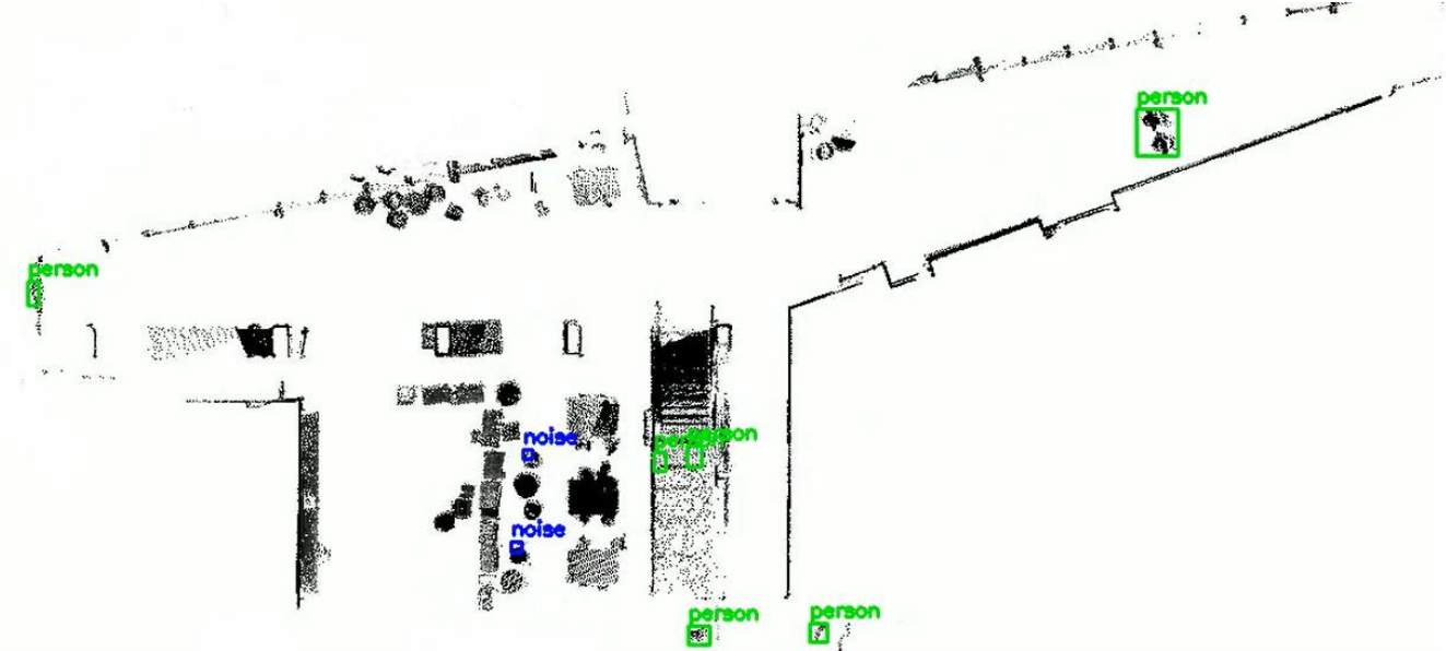
A frame showing people and noise being detected using OpenCV methods in the animations of the lidar stream. The green boxes represent people and the blue boxes represents noise
